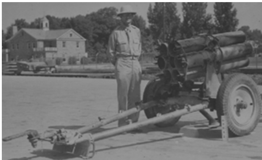
Fig. 2-29. The 150-mm German Nebelwerfer rocket projector was developed in the 1930s; one of its intended uses was to disseminate chemical agents. This fact was supposed to be disguised by naming it the Nebelwerfer (literally “smoke-screen layer”). As events transpired during World War II, Nebelwerfers were used exclusively as rocket artillery, firing high-explosive projectiles. Photograph: Chemical and Biological Defense Command Historical Research and Response Team, Aberdeen Proving Ground, Md.
